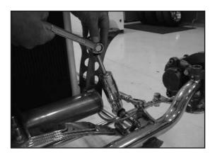
Secure all of the front suspension bolts, making sure they are snug, but not too tight at this time. Torque all fasteners to proper spec at final assembly.
