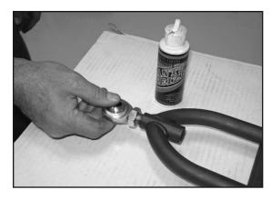
Next, thread jam nuts onto the clevises and screw the clevises into the radius rods. Again, make sure to use anti-seize compound and leave approximately 4-5 threads exposed on each clevis.
