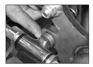
Next, assemble one spring pivot on a batwing. We generally prefer to start with the driver's side pivot. Install the nut on the pivot stud only 4-5 threads at this time. Some applications using our 715-150 shock mount kit may require a spacer as shown to allow adequate clearance between the shock body and the radius rod.
