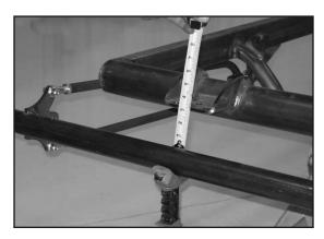
Take measurements to verify that the axle is level from side to side, and that it is positioned approximately 3-inches below the spring perch.
