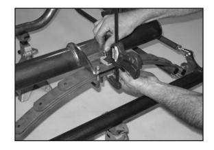
Insert the supplied bushings into the pivot and leaf spring and use the shackle to connect the spring and pivot. On spring behind applications, make sure the shock mount (if used) is on the pivot side of the shackle and that the shackle nuts face forward to prevent interference with the tie rod. Repeat for shackle assembly on the other side.
