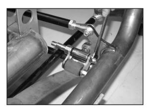
Install shock onto lower mount. It may be helpful to use a little petroleum jelly on the mount to help the bushing slide easier. Secure using the supplied washer and nut.
