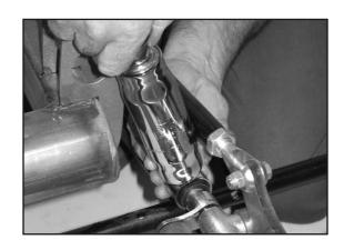
Secure upper shock eye to frame mount. Frame mounts will vary per application (715-150 shock mount shown).
