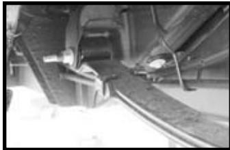
Support the frame with jack stands. The axle should also be supported with jack stands. A jack in the center of the axle will be used to raise or lower the axle when needed.
