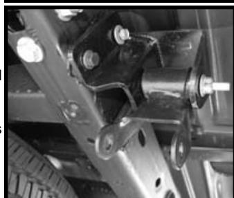
Place the new axle locator bracket on top of the spring with the offset hole to the front of the vehicle. Line up the hole in the bracket with the pin in the spring. Raise the leaf spring and align new bracket under the rear axle. Add a jack stand under the leaf for support.
