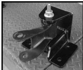
Using the 7/16" bolts provided, bolt the new shackle hanger in the original holes. Install brackets on both sides. Tighten the bolts. Install leaf spring to the shackle. Do not tight shackle bolts until installation is complete.
