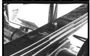
The shackle hanger needs to be removed from the frame on both sides. There is one bolt and three rivets holding it on. There is also a bracket from the bottom of the frame to the shackle bolt. Cut the rivets with a plasma cutter or use a die grinder to slot the rivet and remove with a chisel. The new hanger will reverse the shackle so the spring will mount below. This will lift the truck after flipping the axle.
