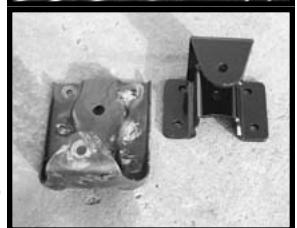
The brake cables are run though a bracket bolted to the frame on the drivers side. Unbolt the bracket.
