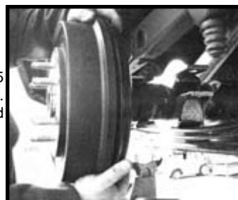
Place the new upper axle plates on top of the axle, align pin with hole on axle. Install the 5/8" bolts provided with one flat washers on top of the upper plate and one on the bottom of the axle locator. Check pinion angle.
