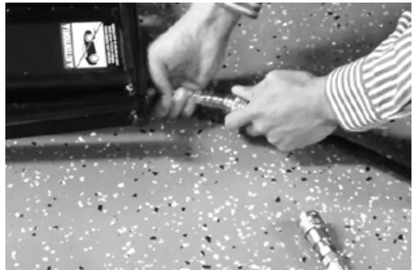
5. For DC Power Units connect directly to a 12-volt power source. Minimum requirement for jumper cables in the USA should be: 7 Gauge. For European countries: 10 square millimeters.
