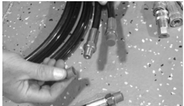
2. Wrap the threads with Teflon tape. When applying tape, wrap it three times in direction shown below.
