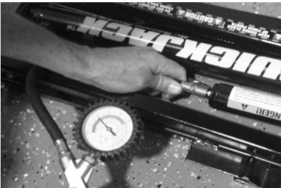
5. Press the air pressure gauge evenly onto the valve stem and record the reading given. If there is a hissing sound, the gauge is not tight or even enough for an accurate reading. **DO NOT EXCEED 50-PSI/3.4 BAR.**
