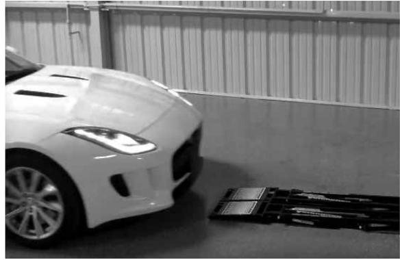
Quick Frame Handles are typically required. They are easily installed by simply lifting the jack frames and placing the end channel underneath the frame tubes as shown here.
