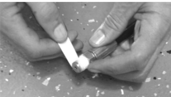
8. Locate the two remaining male quick-connect fittings and attach to Short Leader Hoses as shown below.
