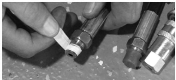
3. Install female quick-connect fitting onto threaded end.
