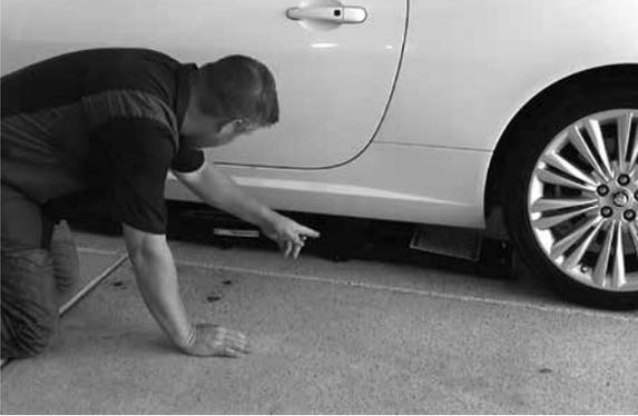
4. When ready, raise vehicle keeping the UP button continuously depressed until tires clear the floor and the jack frames are at least 12" off the ground or the first safety lock position has been reached. **NEVER stop or pause the lift when lower than 12" or first locking position.** The flow divider is inefficient at real high pressures. All scissors lifts on the market are incapable of holding load when less than 7" rise.
