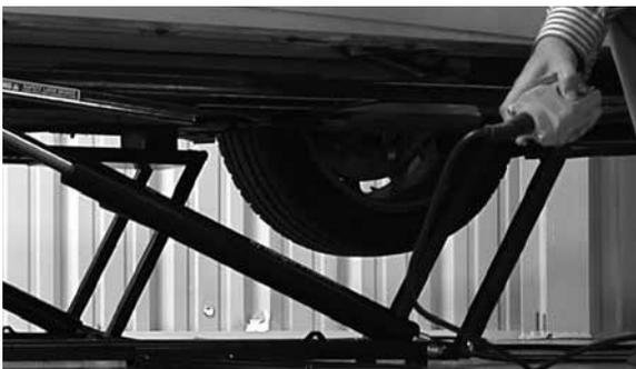
6. Operate the UP control until each jack platform reaches either the low locking position or high locking position.
