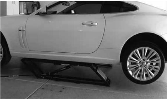
5. Continue to raise to desired height only if vehicle is secure on lift. Keep hair, loose clothing, fingers, and all parts of body away from moving parts. Keep feet clear of jack when lowering. Avoid pinch points.
