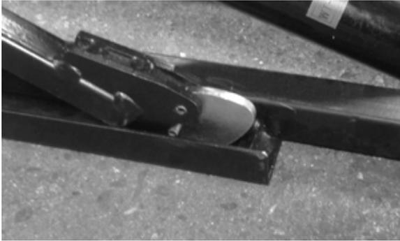
2. Operate the **UP** control until safety lock bars are clear.
