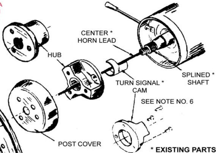
1. Point wheels straight ahead and disconnect battery or pull horn fuse before starting removal of the old wheel so horn won't short out and blow during installation.
