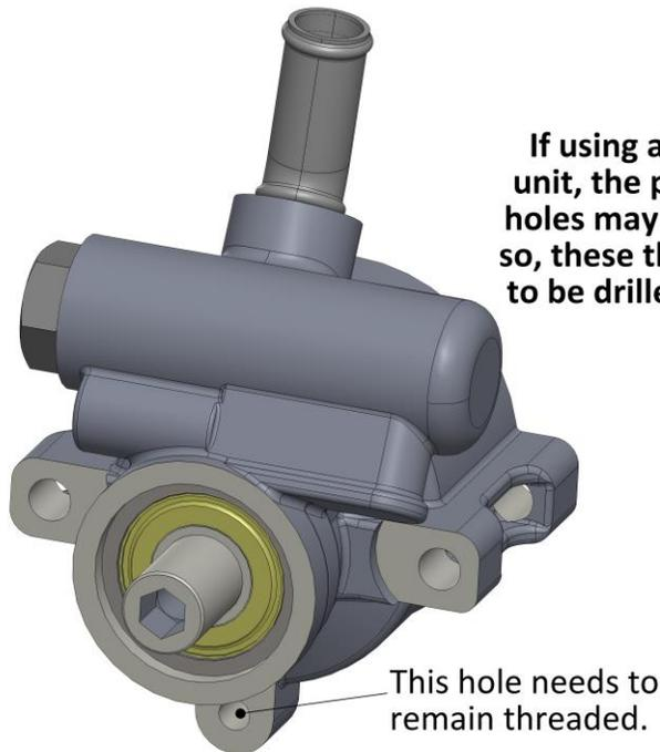
If using a non-Corvette unit, the pump's through holes may be threaded. If so, these threads will need to be drilled out to 5/16".
