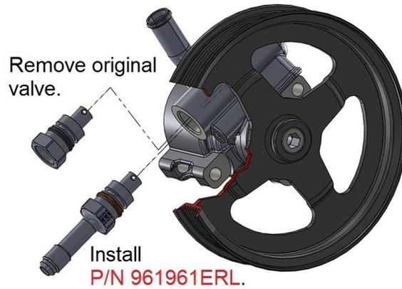
NOTE: If using AN fittings on the pressure line, Holley P/N 961961ERL AN extension/adaptor is required.
