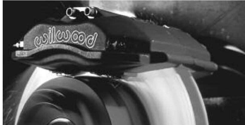
Brake pads bedded on Wilwood's in-house brake dyno
