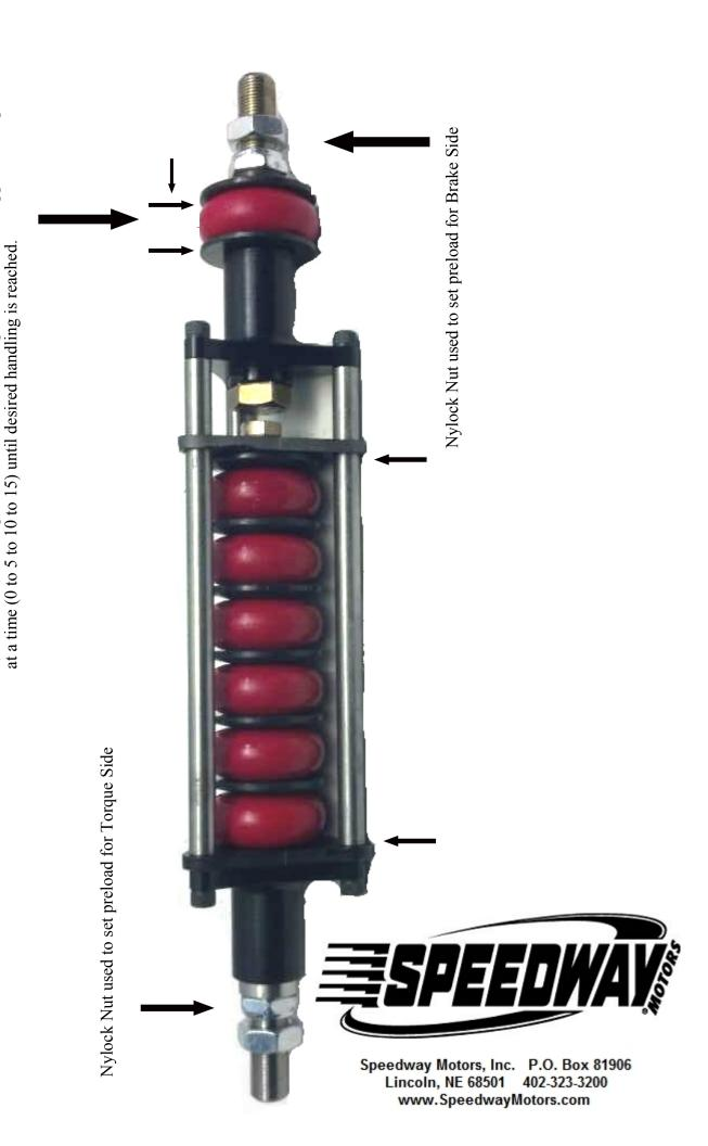
(Brake Side) - To tighten deceleration handling increase washer tapper one step
