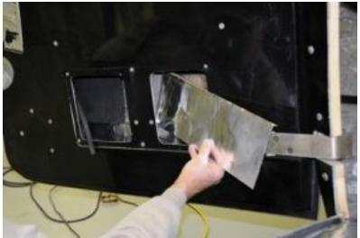
33. The doors were next to be covered on the insides. The 12X23 inch sheets were cut in half for ease of installing them through the small openings in the doors. I was able to install the pieces and then pull the baking paper off inside the doors which worked out fine and keeps them from sticking
