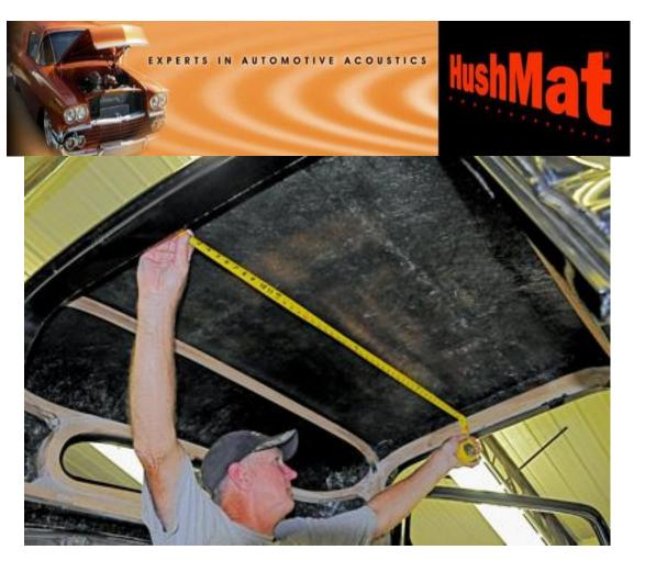
5. The roof area was installed first to eliminate potential damage of the HushMat Ultra sheets on the floor, if installed first. As you can see a measurement of the roof width was taken to find the center.
