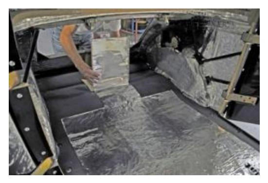
32. The HushMat Ultra sheets were laid all the way to the trunk area in the '32 Ford coupe and the sides were filled in with pieces cut to fit.
