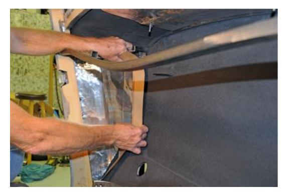
24. Using the same pattern, I merely turned it over or reversed the pattern, to make the piece for the driver side.
