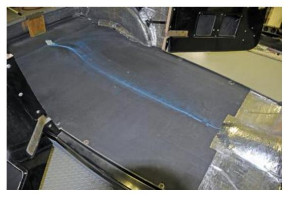
28. The center of the floor was determined next and a chalk line was snapped to mark it.
