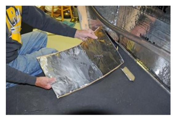
26. The floor is next. The brake pedal arm comes through the floor as most street rods do, so I simply measured where I needed to cut out for it and then slipped the sheet over the pedal arm as shown.
