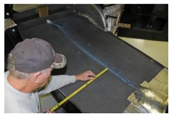
29. Now measure from the center line to determine where the sheets will go to make the best use of all the material and have a neat looking installation.
