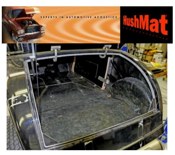
3. The trunk area was open as well so installation was easier. There is no special preparation of the surface needed before installing HushMat. No acetone or other solvent cleaning of the surface was required with HushMat. I vacuumed the complete inside of the body to remove any dirt that was loose on the floor.
