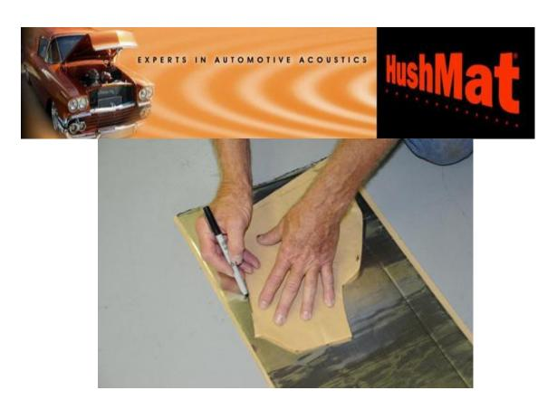
18. After cutting out the drawing made on the backing paper, the pattern is placed on another sheet of HushMat Ultra and traced with a felt tip pen.
