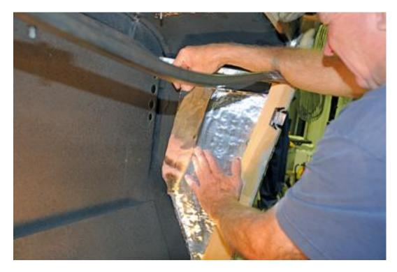
23. The front kick panel area on the passenger side is installed after making a pattern as described earlier.
