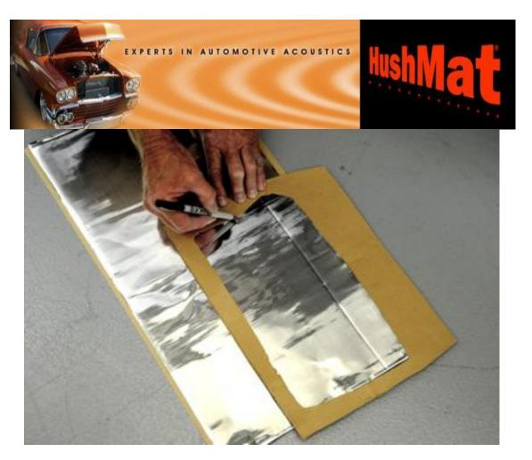
12. Using the template just made, I traced it onto a sheet of HushMat Ultra with a felt tip pen as shown.
