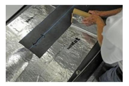
31. The sheets were then laid down along these guide lines. This will produce a very straight and neat installation.
