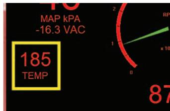
**Coolant Temperature:** The engine coolant temperature is expressed in degrees of Fahrenheit.
