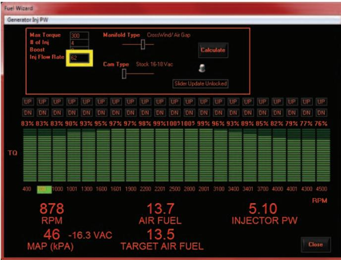
**Injector Flow Rate:** This value will always be 62 unless you have a custom setup with different flow rate injectors. If you have something other than 62 lb./hr. injectors, enter the correct number in this box.
