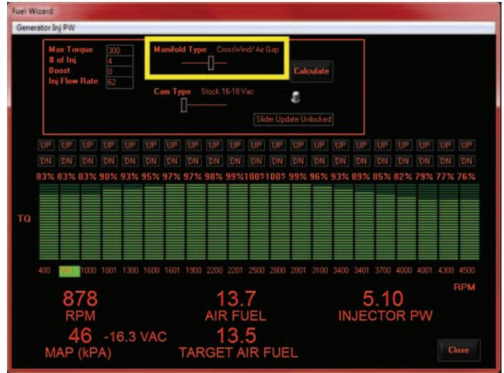
**Intake Type:** Choose from the following: 1. Stock/Cyclone/Performer/Action+Plus, 2. Typhoon/Performer RPM/Stealth, 3. Crosswind/Air Gap, 4. Hurricane/Victor/Super Victor/Team G.
