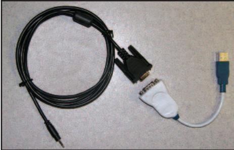
The two cables shown above will allow you to connect your laptop to the Powerjection III.
