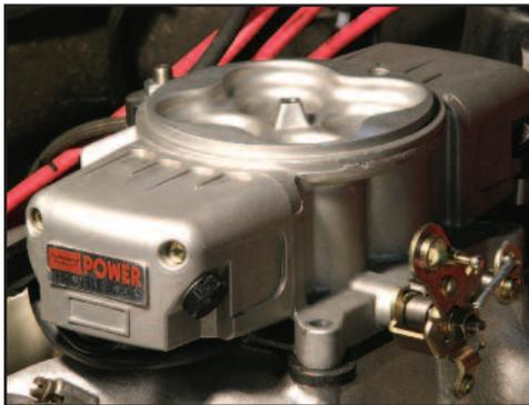
5. **Left** - Install the Powerjection III throttle body assembly onto your manifold. Note: You may need longer carburetor studs. Use Professional Products #20151. Connect your throttle linkage and the throttle return spring. Mount with nuts and washers and tighten. The EMS grounds through the mounting of the throttle body.
