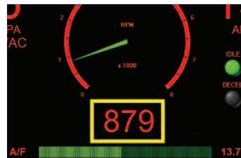
**R.P.M.** This is the large round dial in the center of the screen. It provides both an analog sweep arm and a digital readout.
