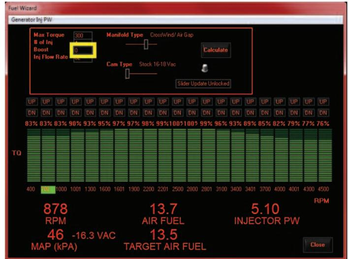
**Boost:** If your engine is normally aspirated (unblown) the value is zero and that is the default. If running a blower, then enter the maximum boost your engine is set up to produce.
