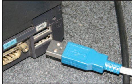
Connect the USB end of the cable to the USB port in your laptop
