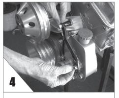
**BOLT ADJUSTING ARM** to front face of pump with stud nut & washers provided.
