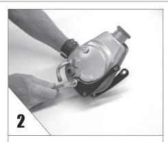
**BOLT REAR BRACKET** to rear bracket to pump using the factory stud.
