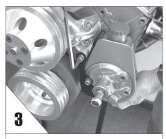
${\bf BOLT\ POWER\ STEERING\ PUMP\ }$  to water pump boss.
