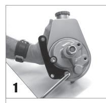
**BOLT** front bracket to the pump. Grind Pump Housing if needed to allow bracket to sit flat on pump boss's. **NOTE**: Bracket must sit flat on face of pump (arrows above show possible points of interference.)
