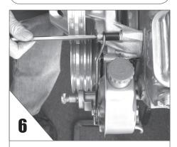
**MEASURE @ PIVOT BOLT** to get the correct length spacer.
