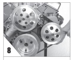
**ATTACH** pulley on pump, install belts as recommended and pull up on pump and tighten nut on adjusting arm.
