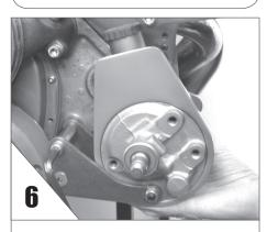
... and **BOLT THE PUMP** to the block as shown and snug up bolts lightly.
