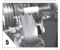
ALIGN pump stud to the adjusting plate...
