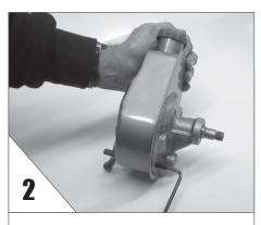
$\mbox{\bf ATTACH}$  the stud to the  $\mbox{\bf FRONT}$  of the pump as shown.
