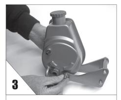
ATTACH the bracket to the pump.
