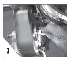
**SWING** the pump back and forth to center the stud in the adjusting slot. When alignment is good, tighten the bolts in the bracket, and the adjusting plate.
