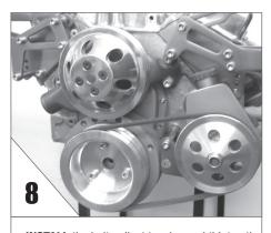
**INSTALL** the belt, adjust tension and thigten the adjusting bolt.
