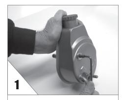
**ATTACH** the **REAR** upper stud to the pump as show.
