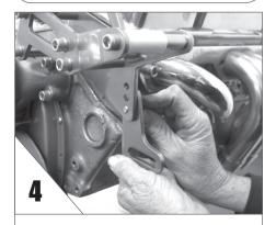
**BOLT** adjusting plate as shown (PIN goes in the middle hole. Bolt is in the bottom hole).
