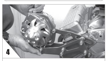
**SWING** the adjusting arm over and hook the 'C' brace to the alternator bottom. **BOLT** the top of the 'C' brace to the alternator as shown.
