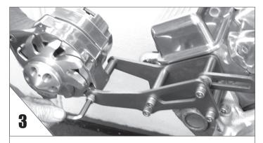
**REMOVE** the white spacer and bolt the alternator in its place. **KEEP** the 1 3/8" spacer in place behind the alternator.
