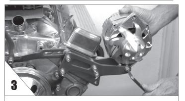
**REMOVE** the white spacer and bolt the alternator in its place.
