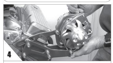
**SWING** the adjusting arm over and hook the 'C' brace to the alternator bottom. **BOLT** the top of the 'C' brace to the alternator as shown.
