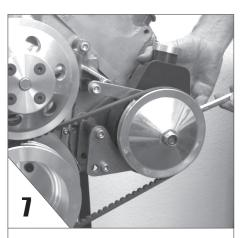
**TIGHTEN** all the bolts and install the belt. Adjust for tension, check that all bolts are tight and the pump is properly aligned.
