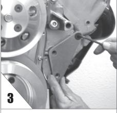
**BOLT** the spacer plate to the block.
