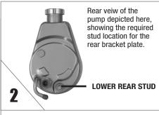
**LOWER REAR STUD** is required for installation.
