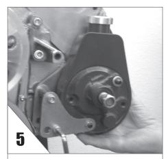
**BOLT** the pump to the block.
