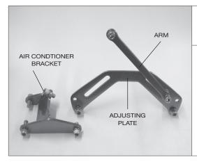
REMOVE the air conditioner bracket and set to the side, keeping the adjusting plate and arm together as shown in the photo.
