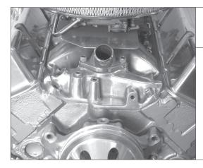
REMOVE the 2 upper water pump bolts.
