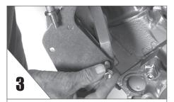
**REMOVE** the nut and plastic sleeve from bracket. Keep bolts and adjusting arm in place. Do not disassemble the bracket.
