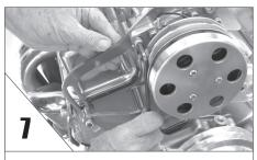
**SWING** the adjusting arm up and bolt it to the compressor with the two bolts. Snug the bolts only for now, not tight.
