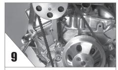
**ADJUST** belt for tension. **TIGHTEN** up all bolts now and check for proper alignment.
