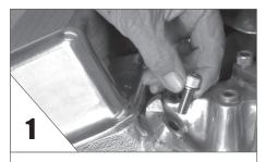
REMOVE the 1st intake manifold bolt.
