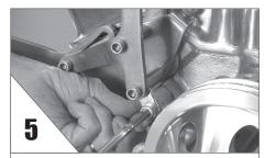
**PUSH** the WPC up to the lower spacer and tighten.
