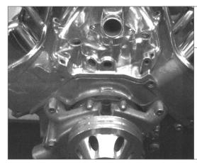
REMOVE the 2 upper water pump bolts.
