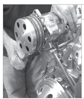
MOUNT the A/C compressor to the bracket.
