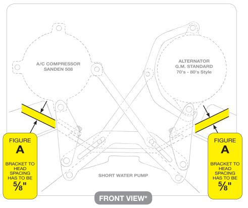
\* VIEW LOOKING AT BRACKET FROM FRONT OF ENGINE COMPARTMENT
