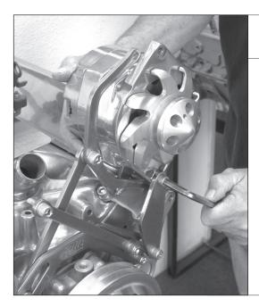
MOUNT the Alternator to the bracket. Make sure the hook on the bottom of the C-Brace is under the alternator.
