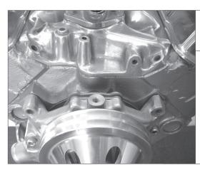
REMOVE the 2 upper water pump bolts.
