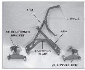
REMOVE the Alternator and Air Conditioner brackets and set to the side as shown in the photo.
