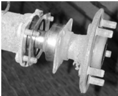
Installation of Spacer Plate.
