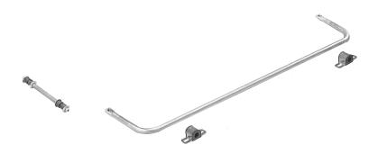
This sway bar is designed to work with the 910-49935 and 910-49942 Composite Leaf Rear Suspension Kits for 1935-40 and 1942-48 Fords.
