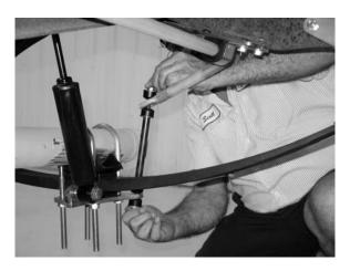
4) Connect top of end link into the eyelet of the sway bar. Connect the bottom of the end link to the leaf spring plate on rear axle assembly. (See note above).
