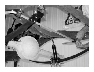
**3)** Install the sway bar on vehicle, securing the retainer straps to the mounting plates with the included hardware.
