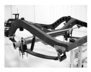
**5)** Lower vehicle to normal ride height prior to tightening all fastener.
