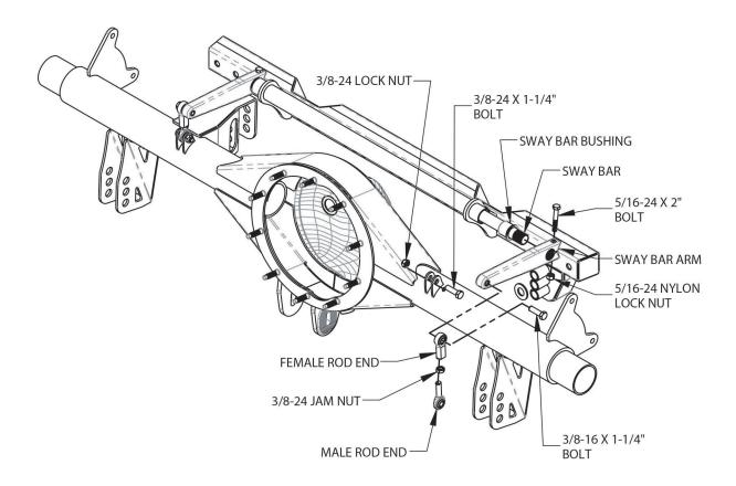
Assemble the opposite side in the same manner. **Note:** Once the vehicle is fully assembled and sitting at ride height on level ground, it is a good idea to disconnect one side of the sway bar links and adjust the length of the rod ends until there is no pre-load and the holes line up perfectly.
