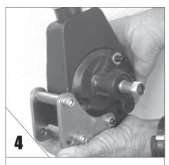
**ATTACH** the bracket to the pump as shown above.
