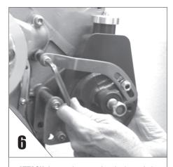
ATTACH the arm by removing the lower bolt and installing the arm as shown. Add washers to keep the arm square with the pump face if needed.
