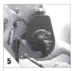
**BOLT** the pump to the block.
