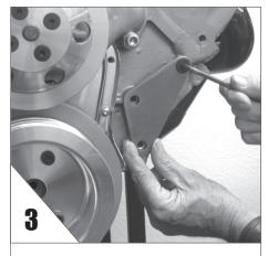
**BOLT** the spacer plate to the block.
