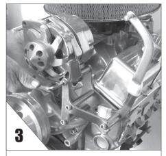
**REMOVE** the white spacer, and bolt the alternator in its place as shown above.
