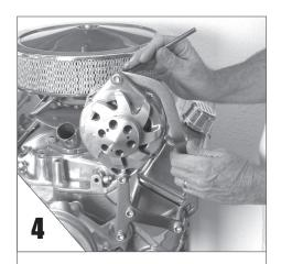
**SWING** the adjusting arm up and bolt the alternator to it with the bolt as shown above.
