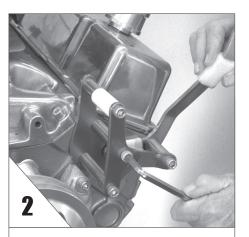
**BOLT** the bracket to the head and snug up bolts. Pivot the adjusting arm out to the side for now.
