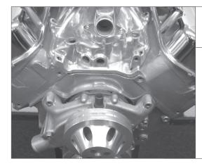
REMOVE the 2 upper water pump bolts.
