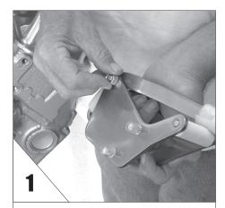
**REMOVE** the nut and plastic sleeves from bolts; keep bolts and adjusting arm in place. Do not disassemble the bracket.
