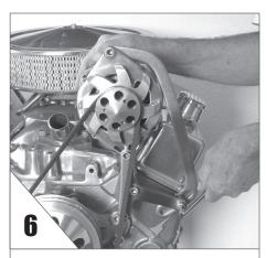
**ADJUST** belt for tension. **TIGHTEN** up all the bolts now and check for proper alignment.
