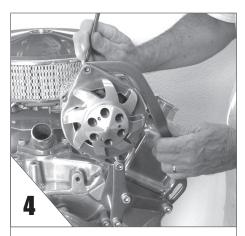
**SWING** the adjusting arm up and bolt the alternator to it with the bolt as shown.
