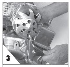
**REMOVE** the white spacer, and bolt the alternator in its place as shown.
