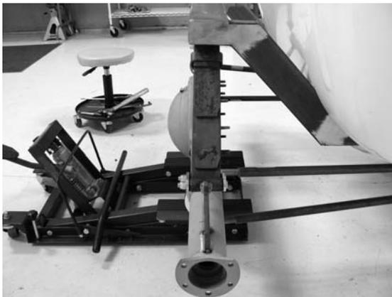
**NOTE:** It is critical that the rear end housing be positioned properly in the chassis prior to installing the spring mounting brackets to eliminate suspension binding and provide a long service life for the shackle bushings. The housing must be centered side to side, perpendicular to the chassis center line, and pinion angle adjusted correctly.
