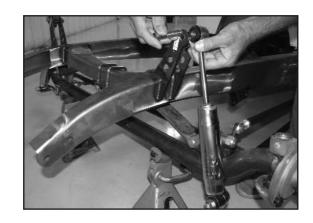
Secure all of the front suspension bolts, making sure they are snug, but not too tight at this time. Torque all fasteners to proper spec at final assembly.
