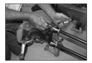
Set the front axle on jack stands under the front of the frame and bolt the clevises to the batwings using the supplied 3/8" x 1" bolts and nuts. Make sure the hardware securing the clevises and rod ends is snug, but not tight at this time. Final torque at assembly should be 20 ft. lb.
