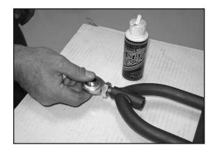
Next, thread jam nuts onto the clevises and screw the clevises into the radius rods. Again, make sure to use anti-seize compound and leave approximately 4-5 threads exposed on each clevis.
