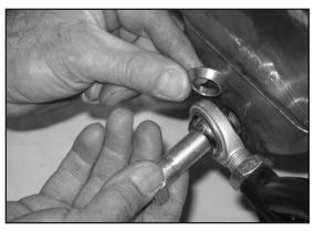
Bolt the radius rods to the frame brackets using the supplied 5/8" bolts and lock nuts. Be sure to use a cone spacer between the frame mount and heim joint to prevent binding. Torque at final assembly should be 100-125 ft. lbs.
