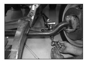
Apply anti-seize to the shank and threads of the spring perch. Install batwing (or wishbone, if so equipped) on axle boss and insert the spring perch. Make sure that batwings are installed on the proper side (they are marked L and R), the ears should be vertical when installed correctly. Install the lower shock mount on threaded shank of spring perch bolt and secure with nut. Do not torque at this time. Torque at final at assembly should be 100-125 ft. lbs.
