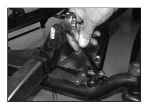
Insert the supplied bushings into the pivot and leaf spring and use the shackle to connect the spring and pivot. Make sure that the shackle nuts face aft to prevent interference with the shock body. Repeat for shackle assembly on the other side, and then tighten spring pivots.
