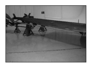
Secure the spring assembly onto the front crossmember or spring perch on the frame using the supplied U-bolts. It's helpful to clamp the spring to the perch while threading the U-bolt nuts on
