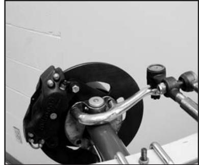
Ford spindle with tie rod ends
