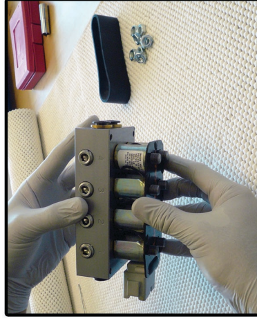
Step 4: Flip the unit upside down and slide the entire coil-pack off of the valve manifold assembly.
