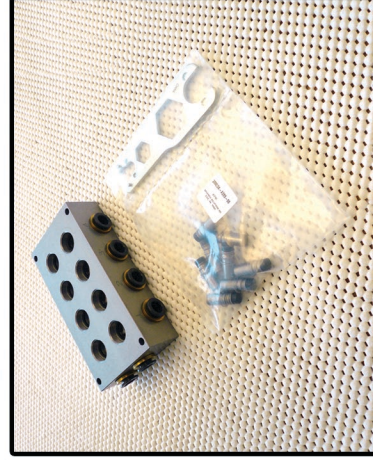
Step 5: With the coil pack separated, now place the valve manifold assembly on a working surface.
