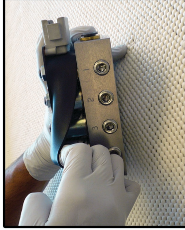
Step 2: Use your fingers to pry the rubber cover off the non-connector side of the coil pack.
