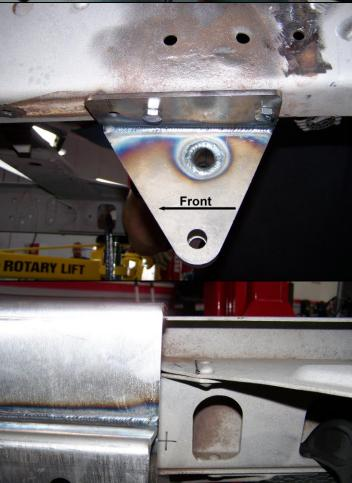
Determining left and right side brackets:
