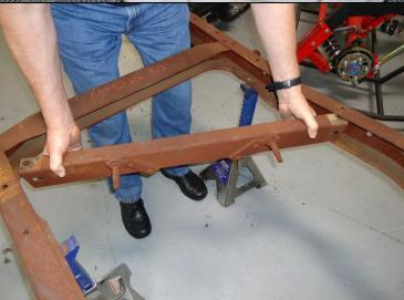
Remove the factory shock cross member using the same process as before with the leaf spring brackets.
