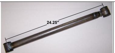
Adjust all the 4-link bars to 24.25" center to center and tighten the jam nuts.
