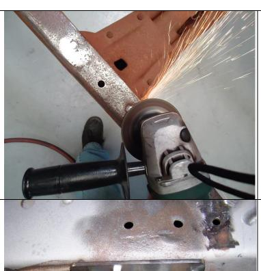
Remove the front leaf spring mounts by grinding off the rivet heads and then punch the rivets body through the frame.
