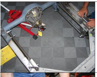
Place a jack under the rear axle. Install the upper 4-link bars onto the upper hole of the axle bracket using the provided 5/8" hardware.
