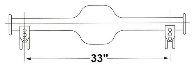
The factory leaf spring pads must first be removed from the housing and the area cleaned up. The axle brackets are installed at 33" Center to center. Make sure that they are centered on the housing. Also, make sure the pinion is pointed up one degree in comparison to the flat area at the backside of the brackets (where the three holes for the coil-overs are located). Use the 3<sup>rd</sup> member mounting face on a Ford 9" or the differential cover on a GM housing as reference.
