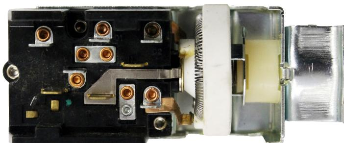
1. Install the new switch into your dash using the original bezel and nut. It will be necessary to cut the shaft for a nice custom installation.
