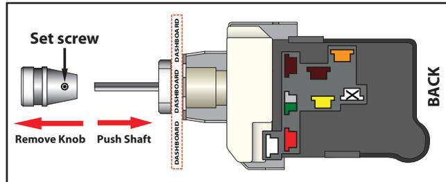
2. Set knob alongside shaft and mark the desired location for cutting on the shaft.
