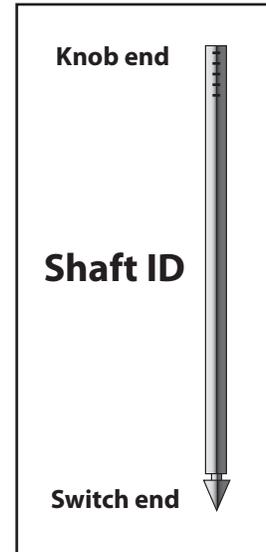
3. Remove the shaft and trim at mark. The shaft can be released from the switch by pulling it outward (toward the rear of the vehicle). Once fully in the "On" position, press and hold the release button on the base of the switch body. Once button is pressed, continue to pull the shaft outward. New switches may be tight, and it might be necessary to move the shaft side to side slightly while pulling to release.
