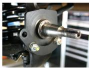
2. With the hardware supplied, install the small bracket to the front side of the spindle using the factory steering arm bolt holes. Install the steering arm at the same time. Tighten down the bracket to the spindle
