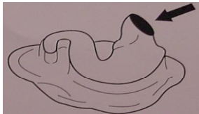
Bad: Canal too Short Foam Stop not deep Enough
