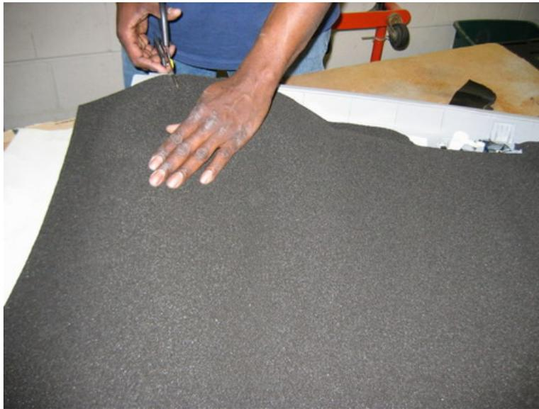
Cut away any foam that overhangs the edges of the door panel with scissors or a utility knife. Hand press the foam to the panel across the surface.
