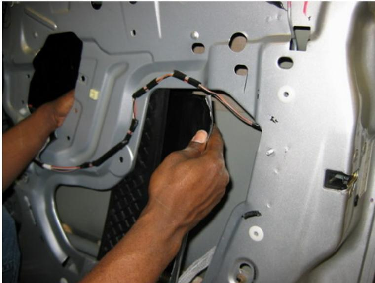
Apply HushMat Ultra Silver or Black Foil damping material to the inside of the outer door skin by removing the brown release paper from the Ultra and passing the sheet through the largest access hole in the frame. Several installers prefer HushMat Ultra black foil as it does not reflect light and will not be seen through speaker grills and other holes in your door.
