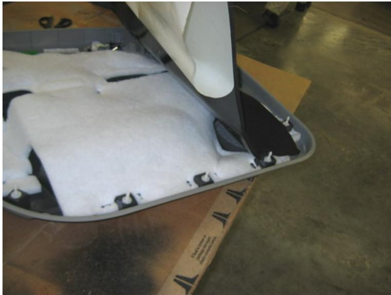
Starting at one straight edge peel back the white release paper and press the sheet onto the straight edge of the door panel. Peel back the release paper completely from the sheet and work around the outer edges of the door panel applying finger/hand pressure to the foam surface.
