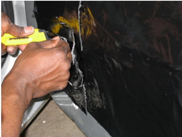
Carefully cut access slits through the HushMat Ultra where wiring or door hardware must pass through. Pull wiring or hardware through slits.
