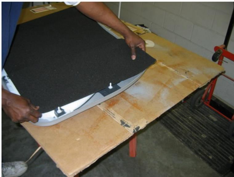
Lay the door panel on a table with the back of the panel facing up. Lay one sheet of Silencer Megabond 1/4" foam against the door panel with the white release paper on the foam. Place the edge of the foam just inside the fasteners or clips that secure the panel to the door.
