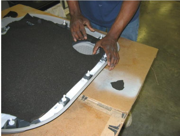
Cut around all panel fastening points, speaker grill, wire harness pass through of any mechanical hardware the will be attached to the vehicle door by slitting the foam and pulling the device through the foam.
