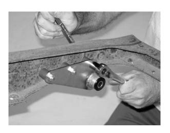
8. Bolt the bracket to the frame using the supplied hardware. Be sure to use the provided sleeves to support the inside of the bracket. NOTE: The left-and right-side brackets look very similar – be sure to use the bracket with the bushing offset to the inboard side of the frame.
