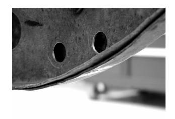
4. The X-member overlaps the frame rail on the inside. Using a 3/4" hole saw with your 1/4" holes as a guide, drill two holes from the inside of the frame through the X-member layer only. DO NOT DRILL THE 3/4" HOLES THROUGH THE OUTSIDE RAIL – ONLY THROUGH THE X-MEMBER LAYER! Afterward, enlarge the holes in the frame rail from 1/4" to 5/16".
