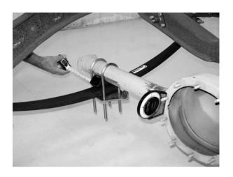
10. Next you need to mock the rearend in place. Put the axle pads on the springs and rest the rearend housing on the pads. Center the housing on the pads and rotate it to achieve the desired pinion angle. When all measurements are verified and deemed correct, the axle pads can be tack welded to the rearend housing. Final welding should be done only after the entire suspension has been trial fit and the pinion angle verified with full weight on the chassis.
