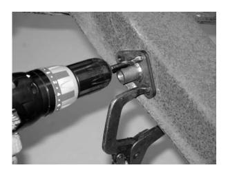
12. Clamp the shock mount to the crossmember with the mount's longest edge parallel to the crossmember's lower flange and the mount sleeve centered on the line drawn in step 11. Use the mount as a guide to drill three mounting holes in the crossmember, and then use the supplied hardware to secure the mount to the frame.
