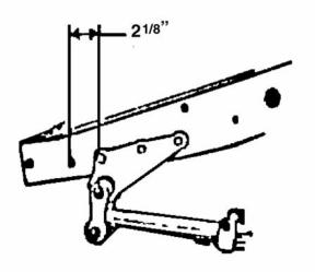
6. To mount the rear spring hanger, begin by measuring 2<sup>1/8</sup>" in from the forward rear bumper mount hole (See Figure 1), and 1" up from the bottom of the rail. This will determine where to drill the rear mounting hole. Slide the bracket onto the frame, making sure it sits flush with the bottom of the rail and the rear bolt hole lines up with the spot you marked. Use the bracket as a guide for marking where to drill the other two mounting holes.
