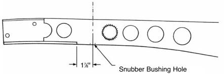
longer spacer to the rear side of the crossmember, using the 5/8" mounting bolts through the crossmember as a guide. Install the gusset horizontally toward the engine between the rear spacer and the crossmember. The rack mounts on the crossmember mount toward the front. Weld the rear spacers and gussets all around. Weld the crossmember spacer in as far as possible inside the crossmember on both sides.
