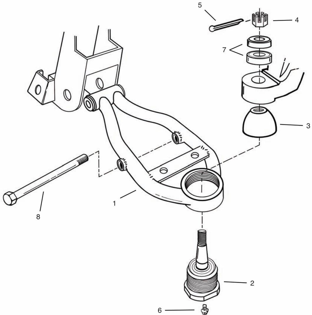
4. Once the car is back on the ground check the position of the lower control arms. The correct ride height is when the lower control arms are level with all the weight on the car. To raise the vehicle ride height turn the adjustment ring clockwise. To lower the vehicle ride height, turn the adjuster counter clockwise. Failure to make this adjustment could result in bent control arms or broken shocks. **NOTE:** All adjustments should be made with the weight off the suspension on jack stands.
