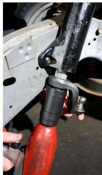
3. Install the new CPP pitman arm to the steering box. It's best to use an impact gun to properly seat the arm on the steering box.
