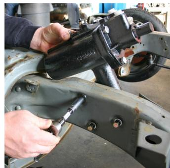
4. Next install the new idler arm on the frame rail.
