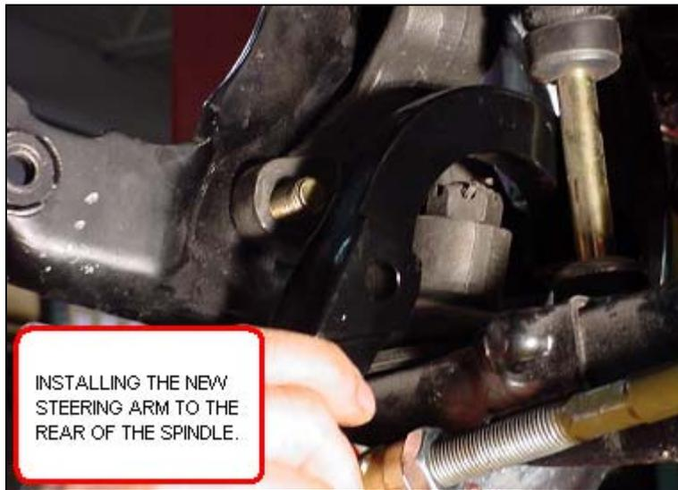
6) Adjust the outer tie rod ends so that each side is on equally (see next page). Insert the outer tie rod stud into the steering arm hole and nut the stud. Torque to **35 ft/lbs.**
