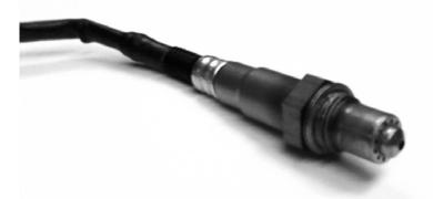
The wideband oxygen sensor needs to be mounted in the exhaust system. A threaded fitting and block off plug are provided. The fitting needs to be welded into place. To install the fitting, drill a .750" diameter hole and weld the fitting centered on the hole. If you do not have access to a welder, any competent exhaust shop can install the fitting for you. Use the supplied block off plug (not your actual oxygen sensor) to cap off your new oxygen sensor fitting until
