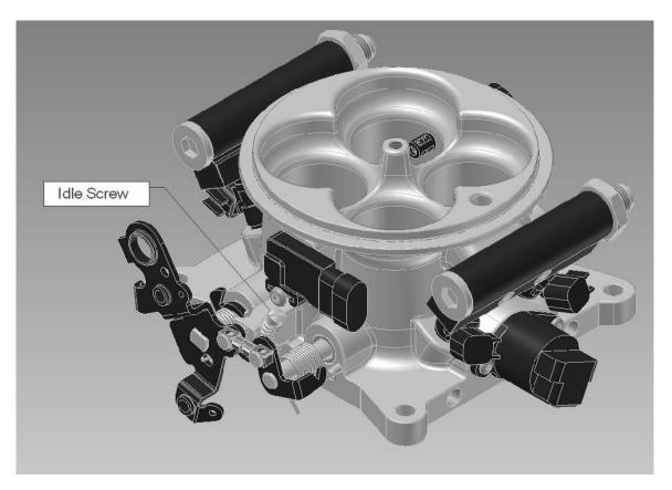
• **TPS IDLE RE-CALIBRATION.** The throttle position sensor is connected to the throttle shaft. So adjusting the resting position of the throttle blades in the previous step may have changed the voltage the ECU is receiving from the TPS. To account for this, you will again be asked to leave the throttle at the idle / closed position and let the ECU capture that voltage.
