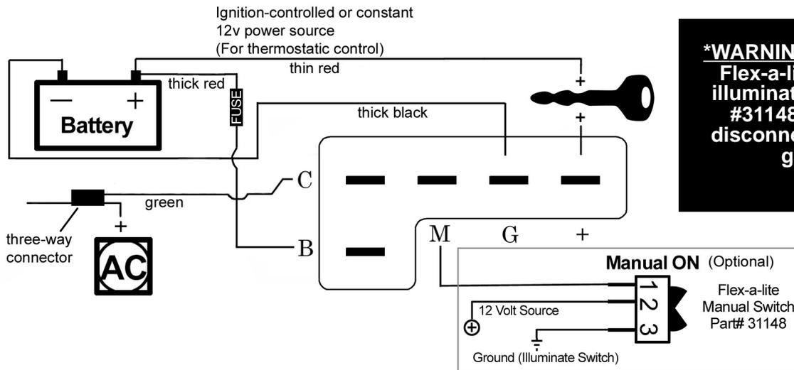
**\*WARNING:** If not using Flex-a-lite's optional illuminated switch (PN #31148), you must disconnect the switch ground.
