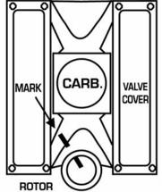
**STEP 5:** Loosen and remove the distributor hold-down bolt and clamp. Lift the old distributor out. If the engine had been running within the past few minutes, the distributor housing may be hot and coated with hot engine oil. Wrap a shop towel around the distributor to avoid burning your hands and dripping oil.
