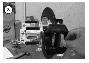
8) Verify that the hub and rotor spin freely with no interference or contact with the caliper. If the caliper is not centered on the rotor use the shims supplied (as required) between the caliper and caliper bracket to center the caliper over the rotor.
