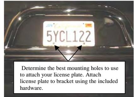
Determine the best mounting holes to use to attach your license plate. Attach license plate to bracket using the included hardware.
