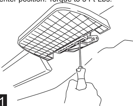
Verify step pad alignment to body line of vehicle.
