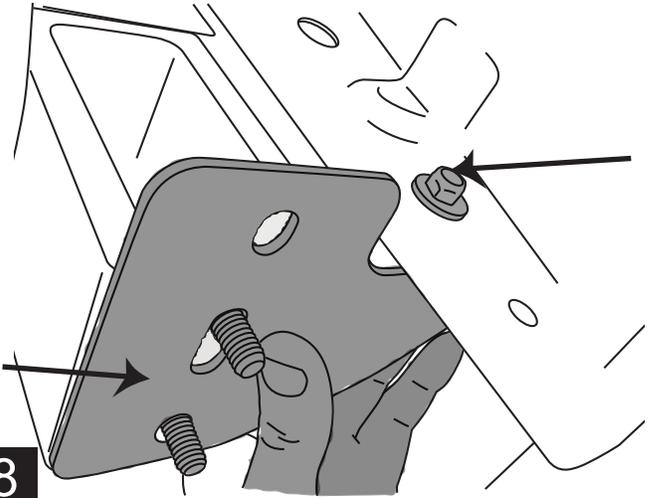
Set linkage into position, tighten bolts using 15mm Socket. Torque to 20 ft-lbs.
