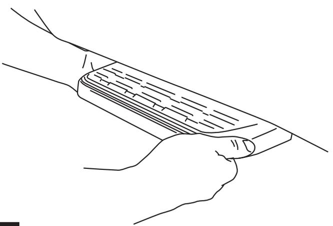
To deploy the step, press down using your foot on the outside edge of the step pad.
