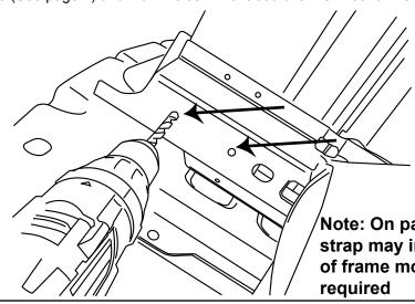
Note: On passenger side Ground strap may interfere with mounting of frame mount. Relocation may be required
