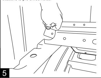
Using a 18mm Socket assemble Frame mount bracket to bed mount bolt. Do not tighten bolts
