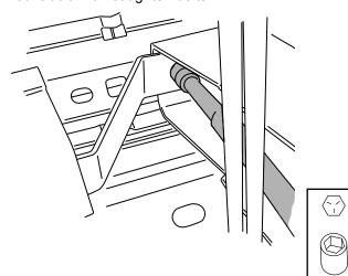
Using 13mm Socket tighten 2 bolts holding Frame mount to bed channel. Do not tighten bolts
