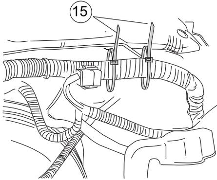
Attach wire harness to the control box. Slide controller through cable ties. Line up cable ties with grooves in controller and tighten.
