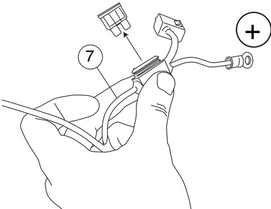
Attach power leads, red lead to positive battery terminal and the black lead to body ground as shown.
