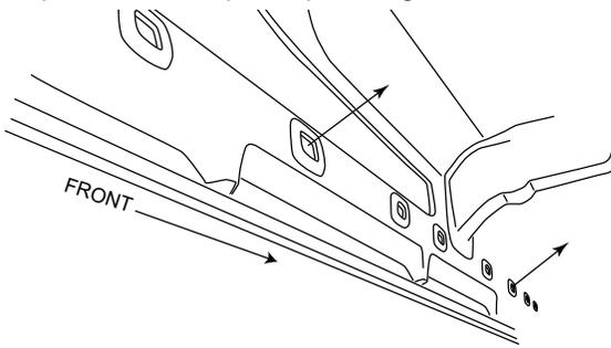
Counting large oval sill holes from the front, remove covering (plug or tape) from the below indicated mounting points.
