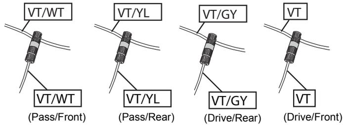
Using supplied Posi-Taps™ splice the Power Step trigger wires into their corresponding door ajar wire. See steps 26 and 27 for wire colors.
