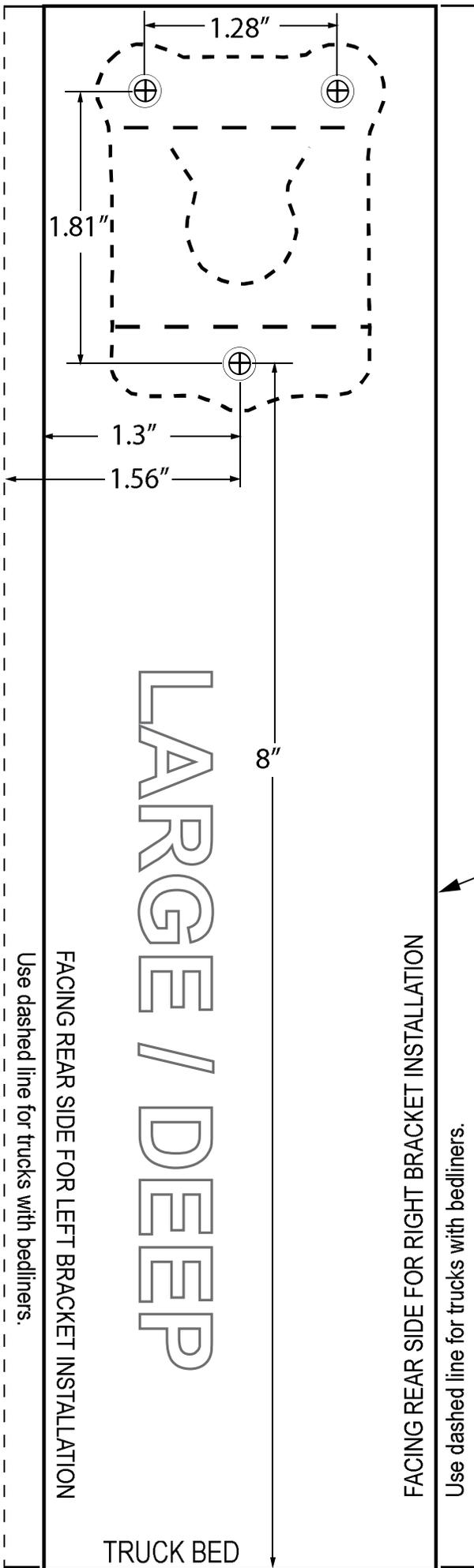
Drill template for BEDXTENDER HD™ mounting brackets
