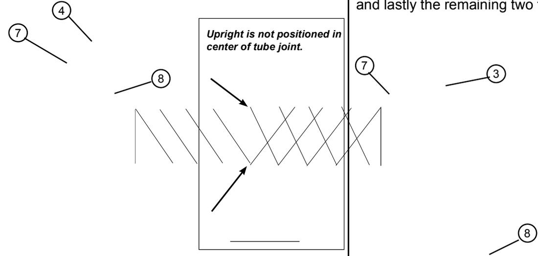
**7** NOTE: The inside of the upright is stepped to fit correctly around the small and large diameter tubes.
