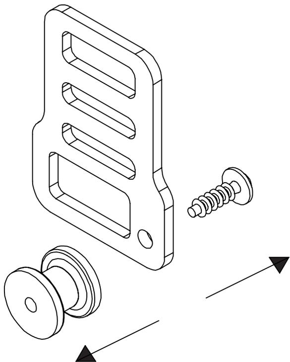
Install Strap Buckle Insert with the provided 10/32 x 7mm socket head cap screw with a 4mm hex key. Repeat for other strap.
