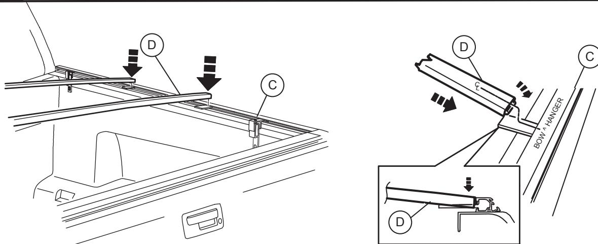
The bow rests upon the top of the clamp with each of its legs draped over the sides.
