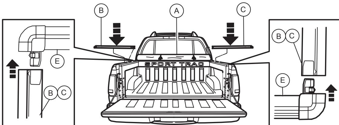
Connect the driver and passenger rails to the front rail. The arrow points to the front of the truck.
