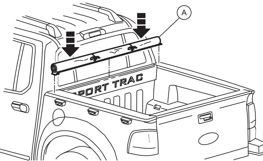
Place the front rail and cover assembly on the top of the truck bed next to the cab.
